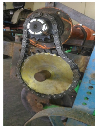
Figure 8: Gear box and shaft power transmission.
