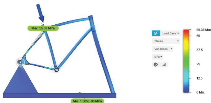
Figure 13: Stress simulation of bike frame and support.
