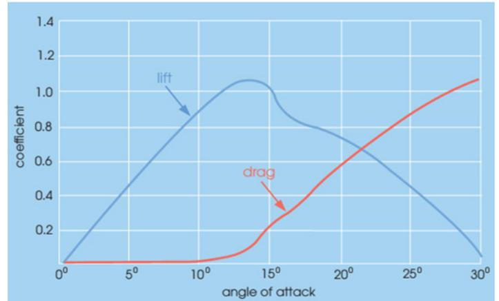
Figure 1: Lift and drag coefficients.
