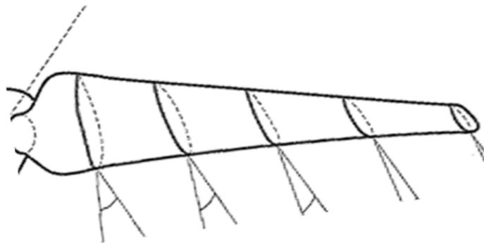
**Figure 9:** angle of twist of different blade sections.
