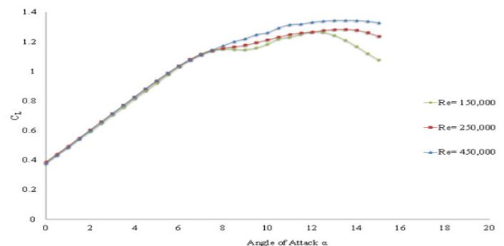
Figure 6: Lift coefficient characteristics of SG6051 aero foil at various angles of attack (aoa) and Reynolds number.
