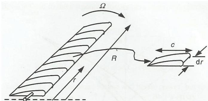
Figure 7: Schematic of blade elements; c, airfoil chord length; dr, radial length of element; r, radius; R, rotor radius;  $\Omega$ , angular velocity of rotor.
