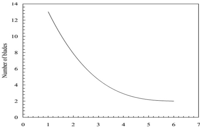
Figure 3: Number of blades and design tip speed ratio.
