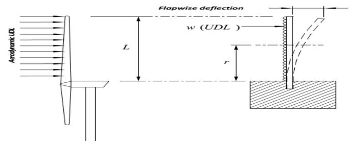
Figure 13: The blade modelled as a cantilever beam with uniformly distributed aerodynamic load.
