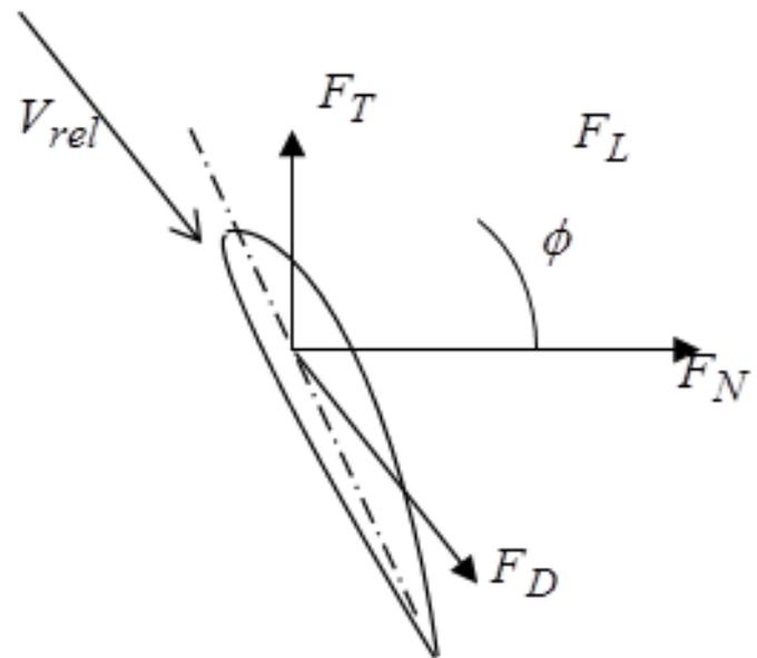
Figure 2: Free body diagram of the main forces acting on air foil.
