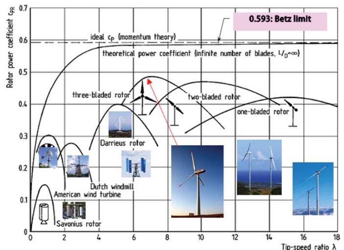
Figure 4: Power coefficient of different wind turbine design configuration.
