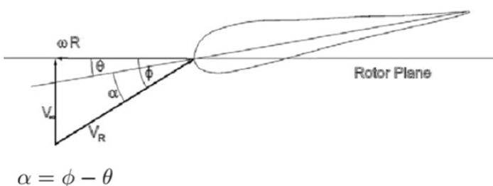
Figure 8: Relative wind speed  $V_{rel}$  has direction  $\varphi = \alpha + \theta$
