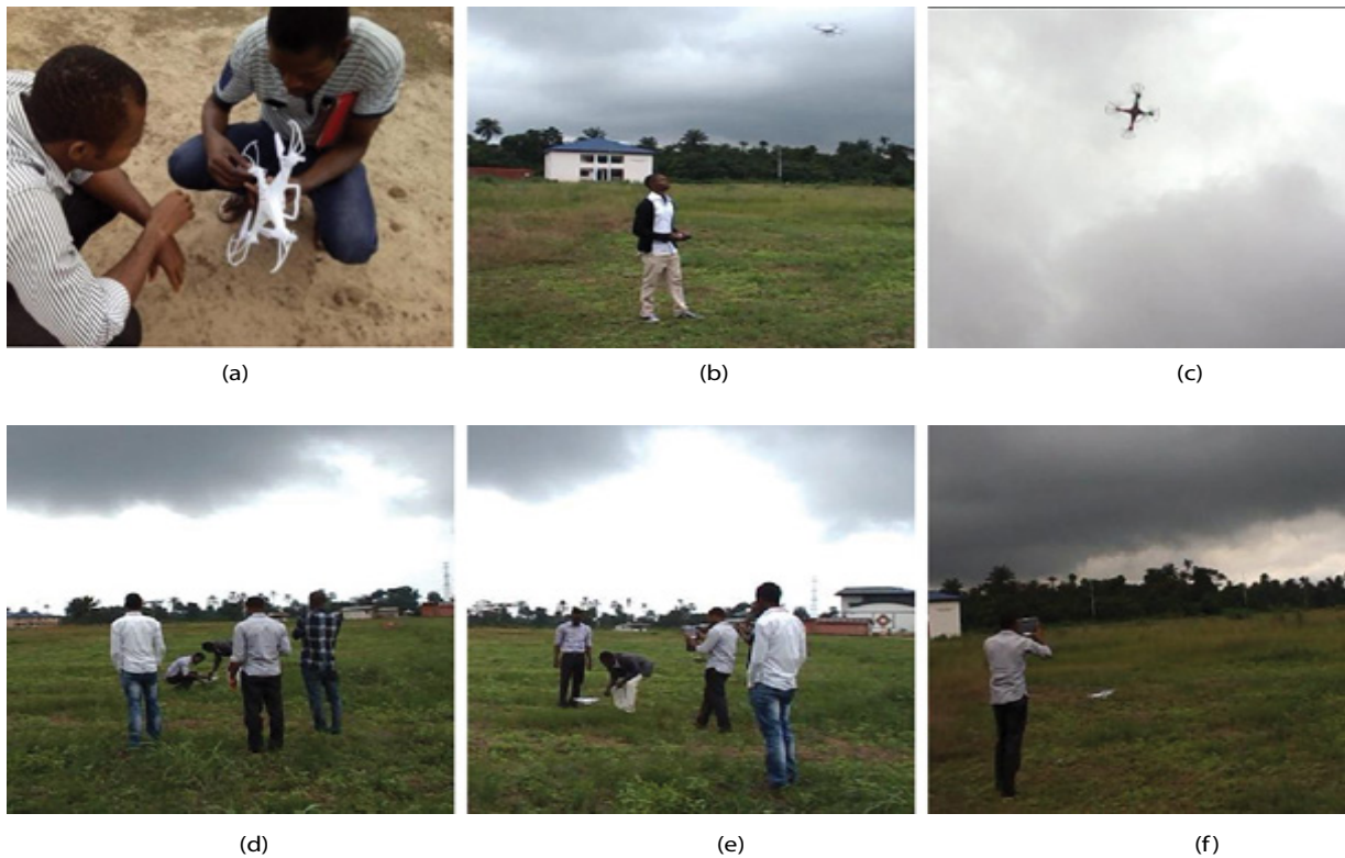
Figure 4: Drug delivery using UAV (a) Loading drug on UAV at base.(b) Controller manning UAV after take-off from base. (c) UAV en route to delivery point. (d) Recipients retrieving drug from UAV at delivery point. (e) UAV departing after delivering drug (f) UAV arriving at home base.
