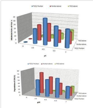
Figure 2: Comparing the three applications for degradation of TOC and COD under different pH values.
