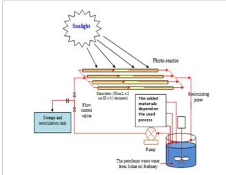
Figure 1: A sketch of the set up for the solar photo-Fenton, solar photocatalyst of  $TiO_2$  and solar photocatalyst of  $TiO_2$ /Fenton process.
