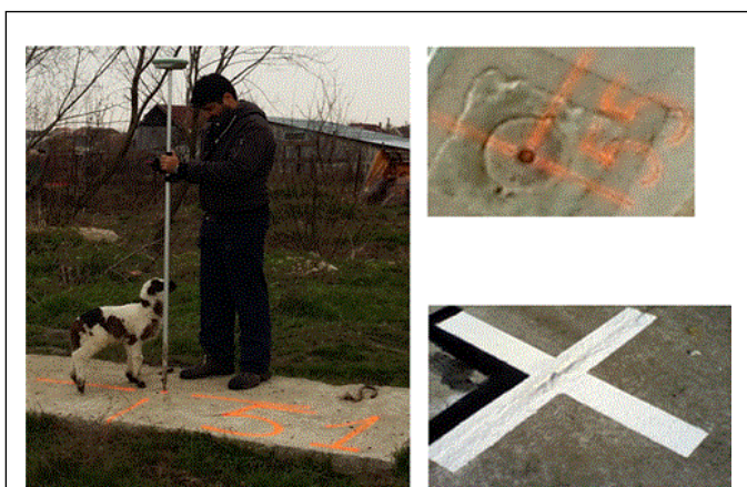
Figure 2: Pre-signaling the control points on the ground.
