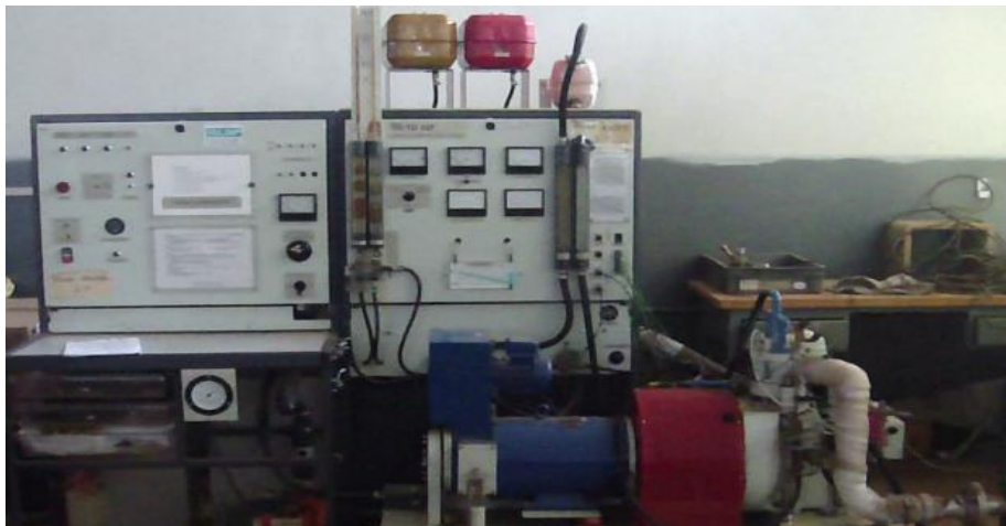
Figure 2.1 TD43F variable compression ratio of engine test rig.
