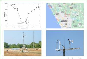
**Figure 1:** Location of the measurement site marked as (\*) in the left panel of the India map. The right panel shows a cityscale map showing location of measurement site (Thumba, blue star).The lower panel shows the eddy covariance system with micro-meteorological sensors used for the present study.
