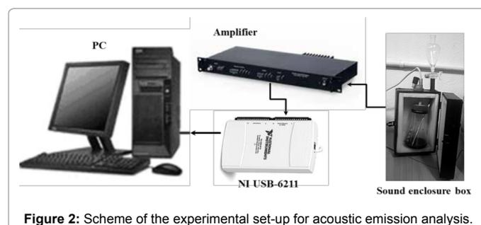
Figure 2: Scheme of the experimental set-up for acoustic emission analysis.
