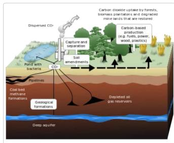
Figure 2: Alternatives for CO<sub>2</sub> sequestration [13] from ref.
