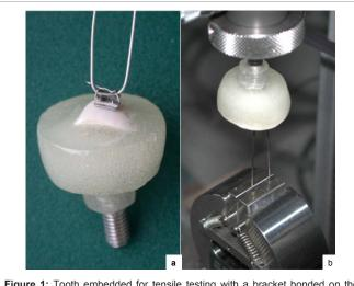
**Figure 1:** Tooth embedded for tensile testing with a bracket bonded on the labial surface and a round steel wire ligated with a stainless steel ligature (a). The samples were mounted on an Instron 4444 (b).
