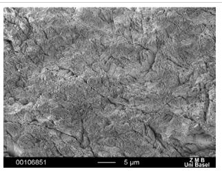
Figure 4: SEM image of an enamel surface after air abrasion with 50 $\mu$  Al<sub>2</sub>O<sub>3</sub> particles and additional etching with 37% H<sub>3</sub>PO<sub>4</sub> for 15 s.
