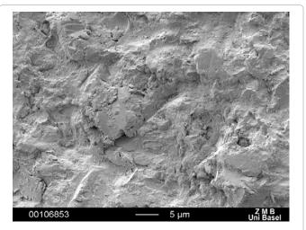
Figure 3: SEM image of an enamel surface after air abrasion with  $50\mu~\text{Al}_2\text{O}_3$  particles.
