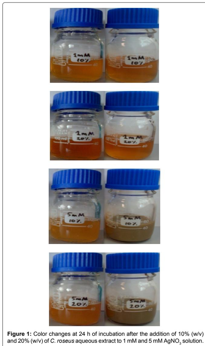
**Figure 1:** Color changes at 24 h of incubation after the addition of 10% (w/v) and 20% (w/v) of *C. roseus* aqueous extract to 1 mM and 5 mM AgNO<sub>3</sub> solution.
