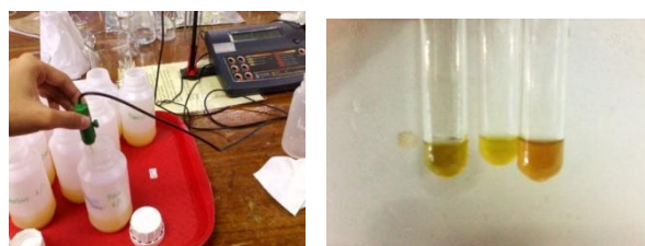
Figure 1d: pH determination from bioethanol for (left), glucose assay (middle)
