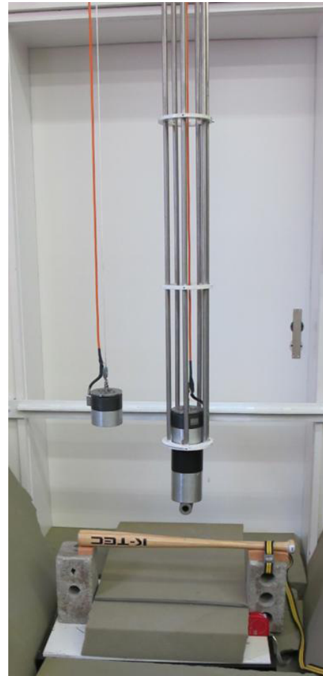
Figure 3: Drop-tower, where the inflicting weapon part was directed to the models.
