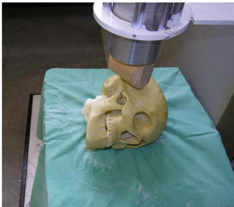
Figure 4: Synthetic skull model targeted by the front part of the baseball bat.
