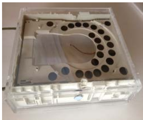
Figure 1: The airtight drawer sampler which was automatically opened and closed in the stratosphere, showing scanning electron microscope stubs onto which stratospheric particles were directly deposited.
