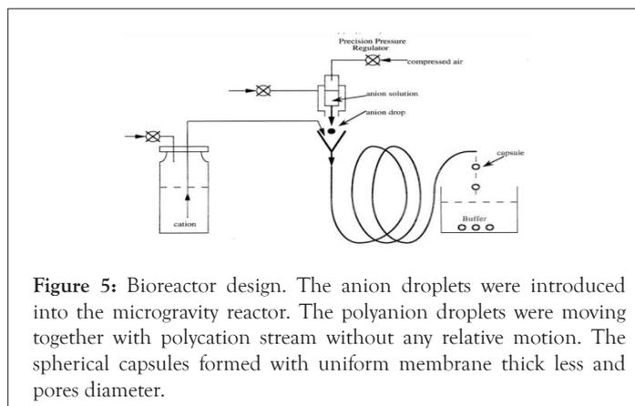
**Figure 5:** Bioreactor design. The anion droplets were introduced into the microgravity reactor. The polyanion droplets were moving together with polycation stream without any relative motion. The spherical capsules formed with uniform membrane thick less and pores diameter.
