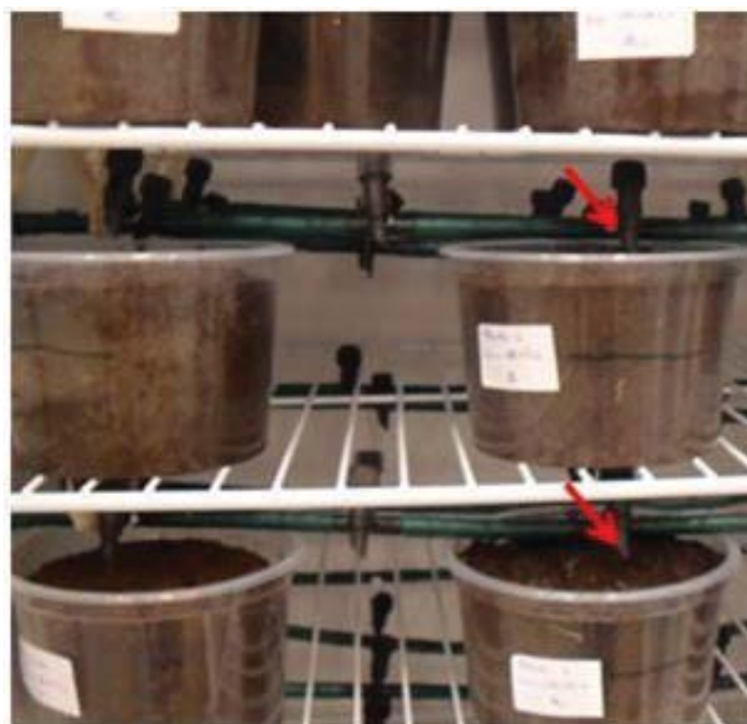
Figure 1: Soil column with drip system indicated by arrow.
