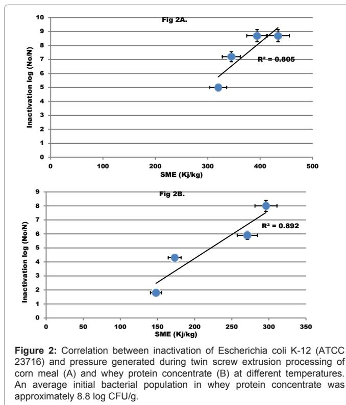
**Figure 2:** Correlation between inactivation of *Escherichia coli* K-12 (ATCC 23716) and pressure generated during twin screw extrusion processing of corn meal (A) and whey protein concentrate (B) at different temperatures. An average initial bacterial population in whey protein concentrate was approximately 8.8 log CFU/g.
