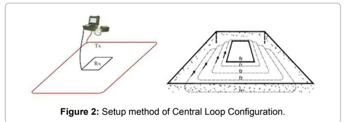
**Figure 2:** Setup method of Central Loop Configuration.
