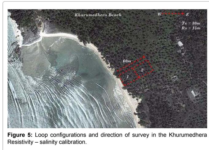
Figure 5: Loop configurations and direction of survey in the Khurumedhera Resistivity – salinity calibration.
