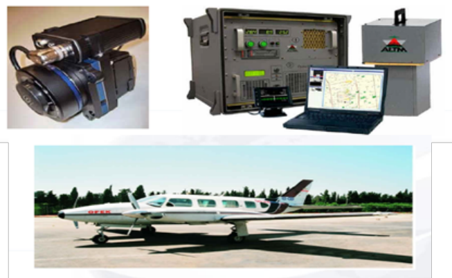
Figure 2: Picture of the ALTM equipment and the Piper Navajo PA-34 air craft
