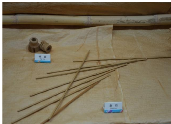
Figure 8: Bamboo is used for the umbrella framework
