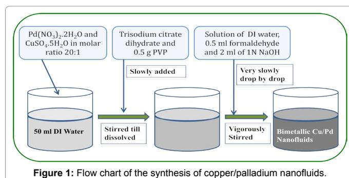
Figure 1: Flow chart of the synthesis of copper/palladium nanofluids.
