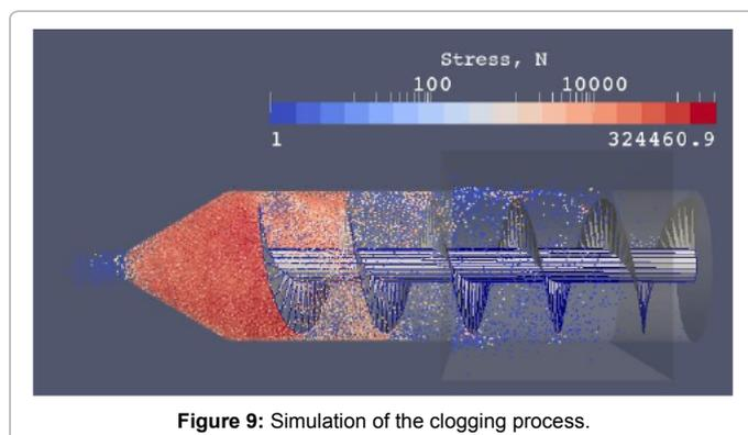
Figure 9: Simulation of the clogging process.
