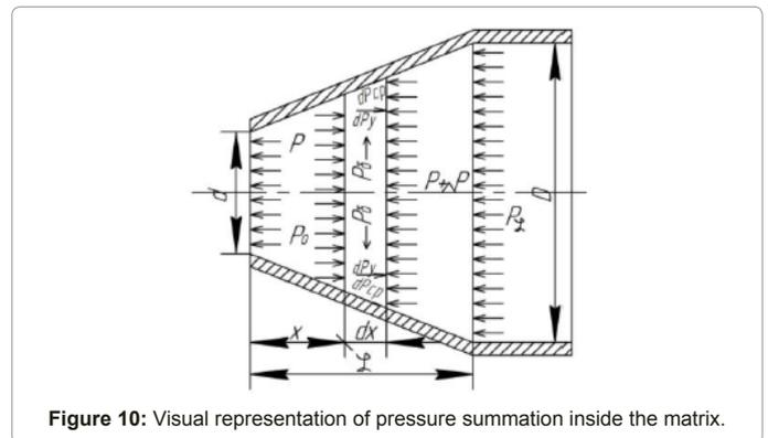
Figure 10: Visual representation of pressure summation inside the matrix.
