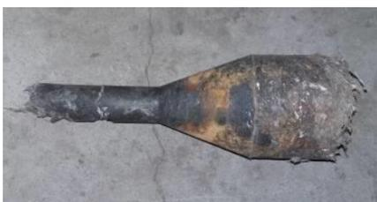
Figure 5: Stopper clog removed from the machine when the frame was cleaned.
