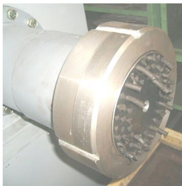
**Figure 1:** Clogged matrices reduce palletising to 50% matrix holes.
