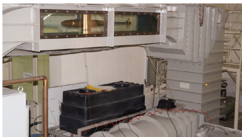
Figure 1: Test section K23 cavitation tunnel.
