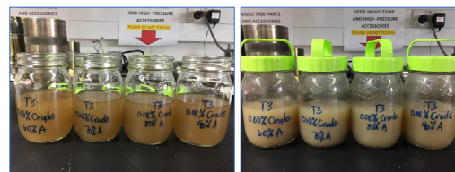
Figure 17a: (A) 0.08% water in oil sample before and (B) after ultrasonication.
