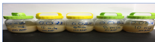
Figure 15: Time optimization of 0.08% oil in water sample by ultrasonication.
