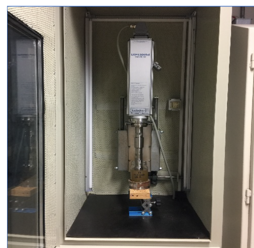
Figure 18: Hielscher ultrasonic device model UIP1500hd in sound proof cabinet.
