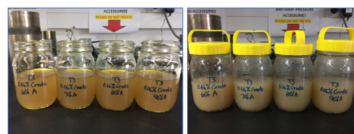
Figure 17b: (A) 0.06% water in oil sample before and (B) after ultrasonication.
