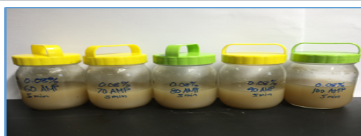
Figure 16: Amplitude optimization of 0.08% oil in water sample by ultrasonication.
