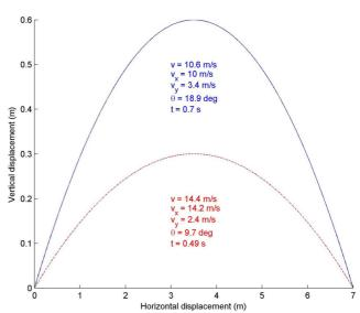
**Figure 2:** Theoretical trajectories and corresponding initial conditions for projectiles with the same maximum horizontal displacement (7 m) but different maximum heights. The maximum vertical displacement of the solid (blue) trajectory and the dashed (red) curve are 0.6 m and 0.3 m, respectively.
