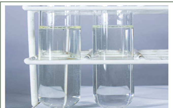
Figure 2: CTAC colloidal solution (left) and W/W emulsion (right) consisting of HCl emulsified in (P44414) Cl.
