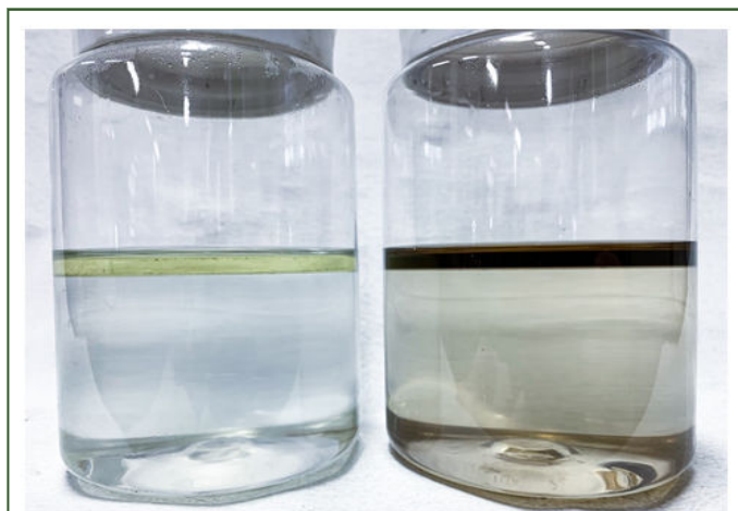
Figure 4: Failed attempts to mix HCl in (P44414) Cl (W/W) emulsion. Left: No emulsifier was used; Right: Only PEG 400 DO tested as emulsifier for the W/W emulsion. The layer on top of both experiments is the (P44414) Cl.
