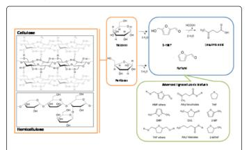
**Figure 1:** General scheme for the transformation of lignocellulosic biomass into advanced oxygenated biofuels.
