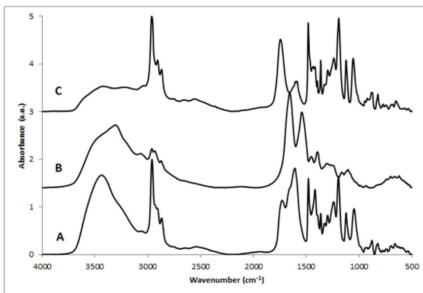
**Figure 5:** (a) Analysis of UV-Vis spectra (230–590 nm) of Mb *c* in 50 mM phosphate buffer pH 6.5, Mb *c*–<sup>1</sup>Butyl[6]CH<sub>2</sub>COOH complex in CHCl<sub>3</sub> and Mb *c* in aqueous phase after the extraction process with calixarene. (b) FTIR spectra of (A) Mb *c*–<sup>1</sup>Butyl[6]CH<sub>2</sub>COOH complex, (B) free Mb *c* and (C) <sup>1</sup>Butyl[6]CH<sub>2</sub>COOH.
