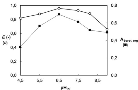
**Figure 4:** The effect of pH<sub>ini</sub> of aqueous solution of 14.7 μM Mb *c* on the degree of extraction ( $E$ ), with 3 mM<sup>t</sup>Butyl[6]CH<sub>2</sub>COOH in CHCl<sub>3</sub>. E(-)(○); A<sub>soret,org</sub>(■).
