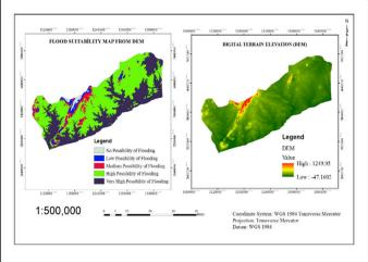
Figure 4: Digital Terrain Model and its associated flood suitability map.
