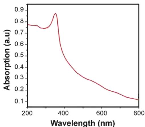
Figure 5: UV-Visible absorption spectrum of ZnO nanofluids.
