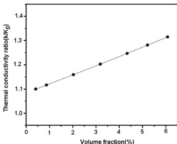
Figure 6: Thermal conductivity ratio as a function of ZnO volume fraction.
