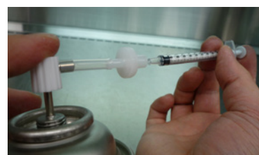
Figure 4: Flushing a syringe with nitrogen gas. Syringe is flushed 5 or more times with nitrogen gas to remove the air. After assembly with needle, nitrogen is ejected from the syringe through the needle.
