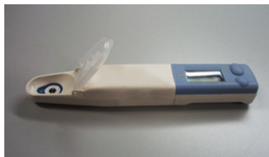
Figure 5: Compact pH meter. As for the medium sealed in a vial, the pH is measured using the compact pH meter in small volumes.
