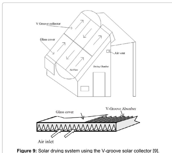
Figure 9: Solar drying system using the V-groove solar collector [9].
