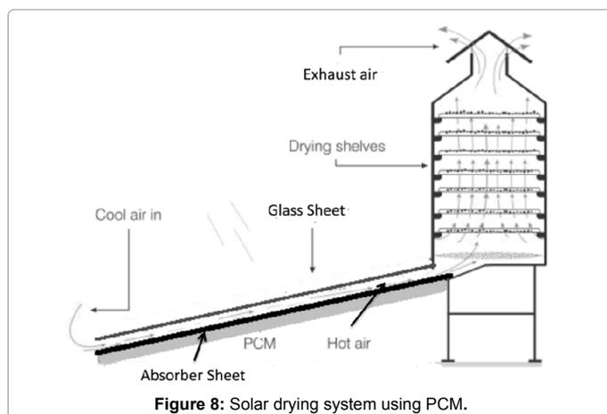
Figure 8: Solar drying system using PCM.
