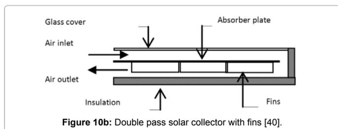
Figure 10b: Double pass solar collector with fins [40].
