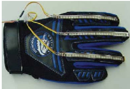
Figure 2: Low-cost visual motion data glove
