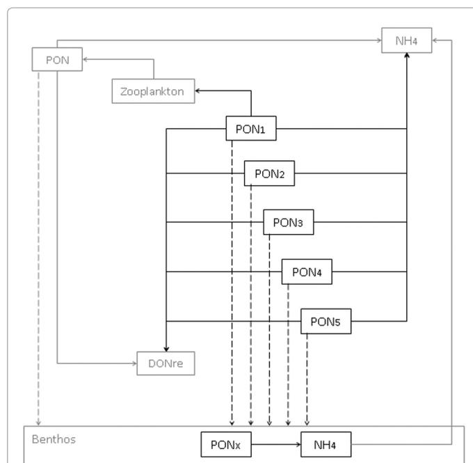
Figure 2: Scheme of the modelled nitrogen and phosphorus pools; for simplicity, only the nitrogen pools are represented. Arrows denote the processes that link the different components of the algorithm. The structure and processes from the basic setup of the Mohid Water Quality module are represented in dark gray, whereas the adapted processes for the POM pools simulation are represented in black. Sinking rate is represented by the dashed arrows. PONx stands for all PON pools.
