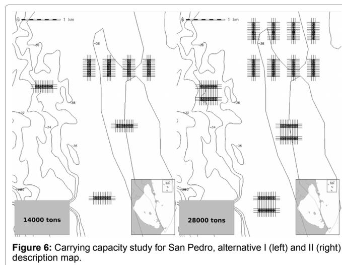
**Figure 6:** Carrying capacity study for San Pedro, alternative I (left) and II (right) description map.
