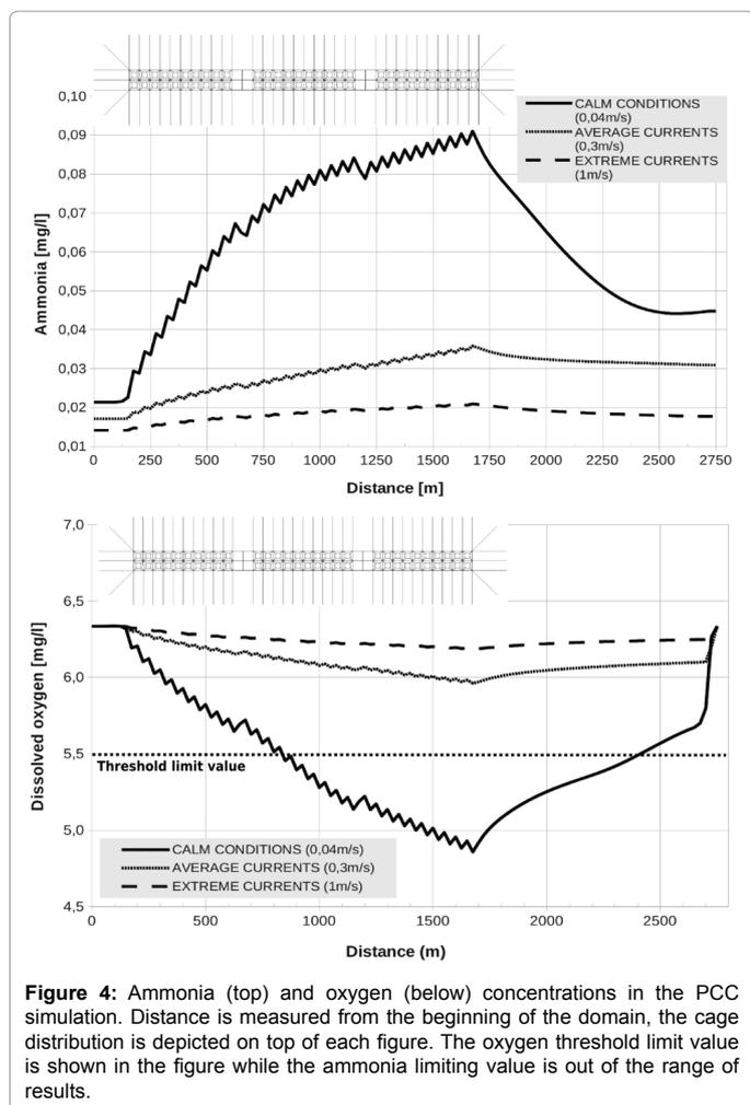
**Figure 4:** Ammonia (top) and oxygen (below) concentrations in the PCC simulation. Distance is measured from the beginning of the domain, the cage distribution is depicted on top of each figure. The oxygen threshold limit value is shown in the figure while the ammonia limiting value is out of the range of results.
