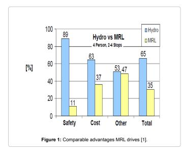
(Figure 1). Though having a higher initial cost MRL systems are more suitable for use than conventional system. F Celik concludes by stating that in the near future elevator market will be dominated by MRL and hydraulic drives sharing a majority of the market share.
