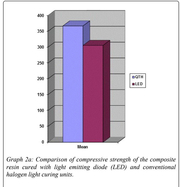
Graph 2a: Comparison of compressive strength of the composite resin cured with light emitting diode (LED) and conventional halogen light curing units.
