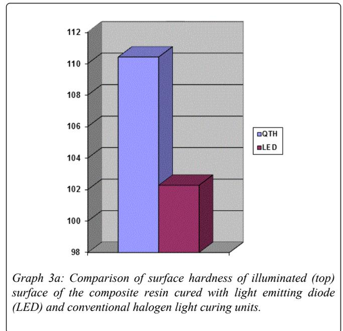
Graph 3a: Comparison of surface hardness of illuminated (top) surface of the composite resin cured with light emitting diode (LED) and conventional halogen light curing units.
