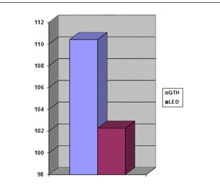
Graph 3a: Comparison of surface hardness of illuminated (top) surface of the composite resin cured with light emitting diode (LED) and conventional halogen light curing units.
