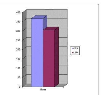
Graph 2a: Comparison of compressive strength of the composite resin cured with light emitting diode (LED) and conventional halogen light curing units.
