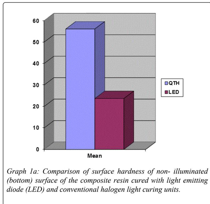
Graph 1a: Comparison of surface hardness of non- illuminated (bottom) surface of the composite resin cured with light emitting diode (LED) and conventional halogen light curing units.
