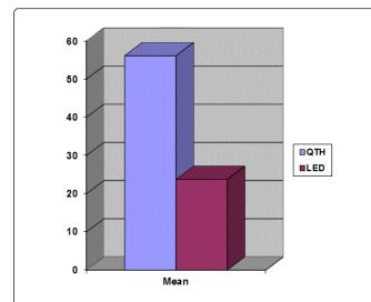
Graph 1a: Comparison of surface hardness of non- illuminated (bottom) surface of the composite resin cured with light emitting diode (LED) and conventional halogen light curing units.
