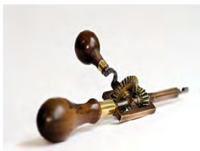
Figure 2: Archimedean drill, 19 th century [6] REF by 1611 century practitioner [3]. British dental association museum/science photo library, C009/8255 rights managed.
