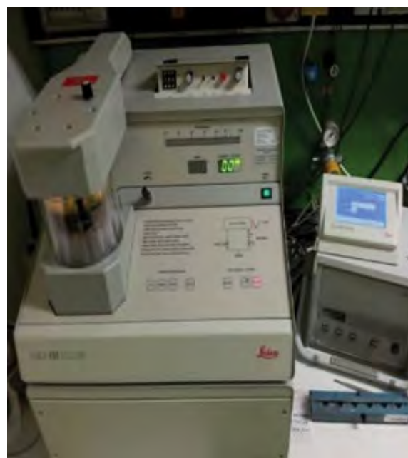
Figure 37: Gold coating machine.
