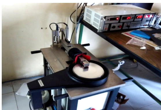
Figure 1: Pin on disc wear testing machine.
