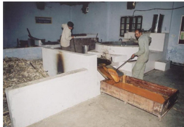
Figure 1: Triple pan furnace in operation.
