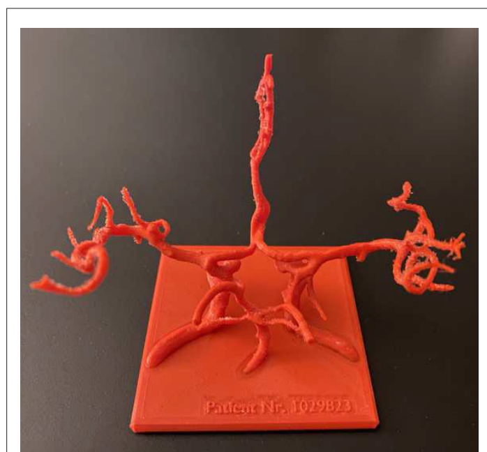
Figure 4: 3D printed 1:1 model of the cerebral vasculature in red polylactic acid PLA after dissolving polyvinyl alcohol PVA support.
