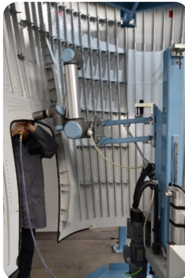
Figure 1: Collaborative riveting process between humans and robots at ZeMA.
