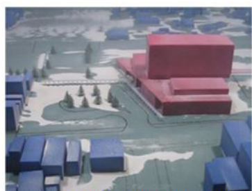
Snow & wind simulations using wind tunnel
