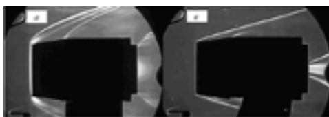
Figure1: Nozzle startup experiment: a - unsuccessful startup if the nozzle is installed before the start of blow down, b - a successful starting if the nozzle is thrown into the airflow at Mach number of 6.
