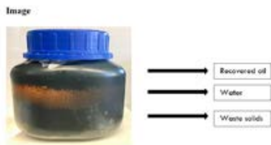
Figure 1: Separated phases in oily sludge after centrifuging with the effects of additives and pre-heating.
