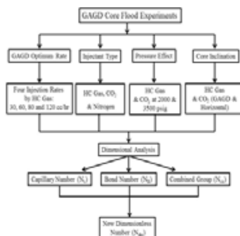
Figure 1: Experimental design and dimensional analysis scheme during high pressure gravity assisted flow.
