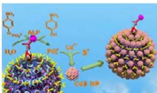
Figure 1. Microbead linked enzymatic generation of CdS nanoparticles.
