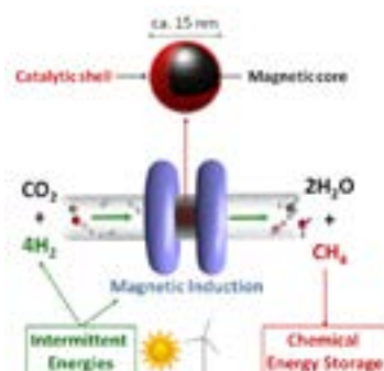
Figure 1: Illustration of the concept of chemical energy storage through magnetic induction.
